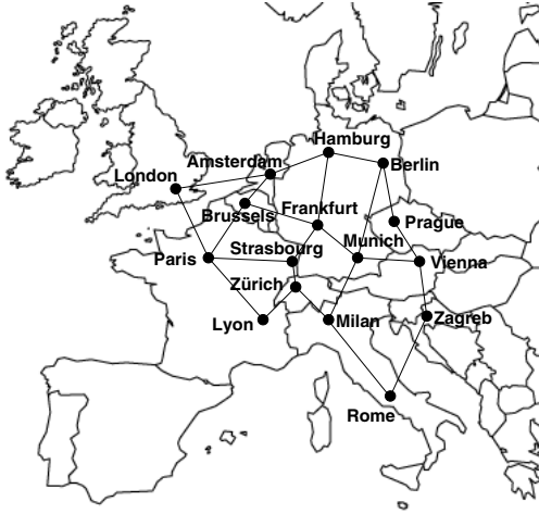
Fig. 1 Pan-European Network Scenario [4] total traffic = 1 Tbps, mean number of \lambda s/link = 5.43
