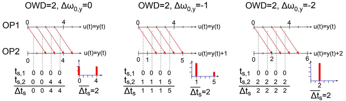
**Figure 4.23:** Impact of resolution offset due to system clock skew on error distribution
