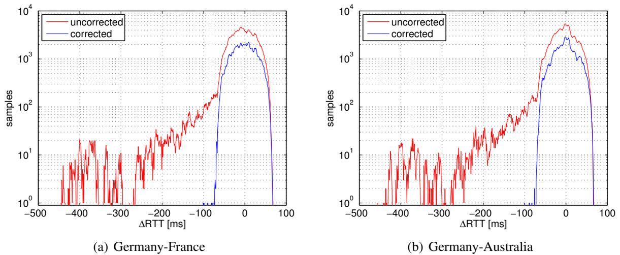
**Figure 7.5:** Difference between RTT from active measurement and flow-based OWD
