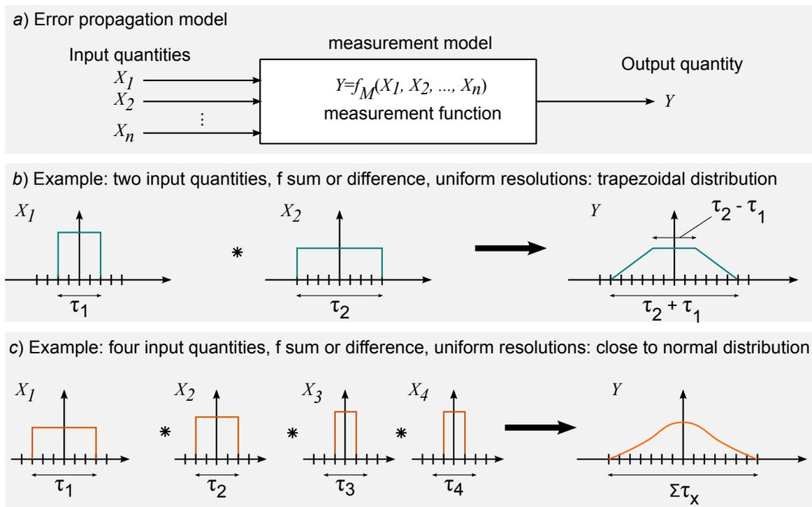
**Figure 2.8:** Error propagation in a measurement system
