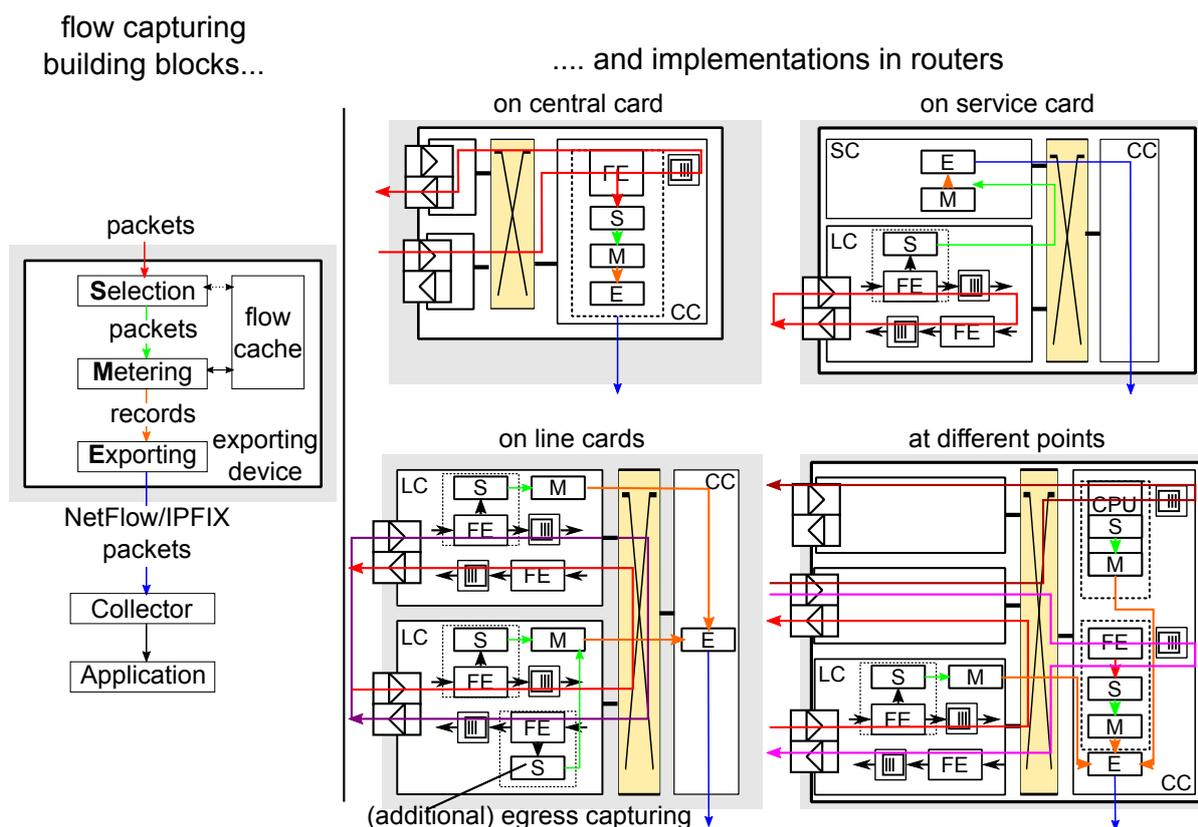
**Figure 3.16:** Flow capturing: building blocks and points for implementations in routers
