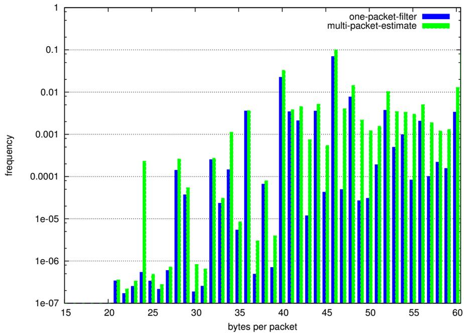
**Figure A.1:** Packet size distribution histograms. Truncated at 60 bytes, logarithmic Y-Axis.
