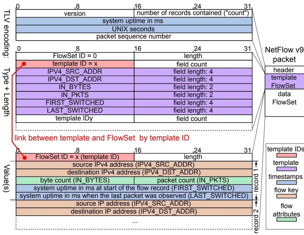
**Figure 3.14:** NetFlow version 9 packet format (exemplary template shown)
