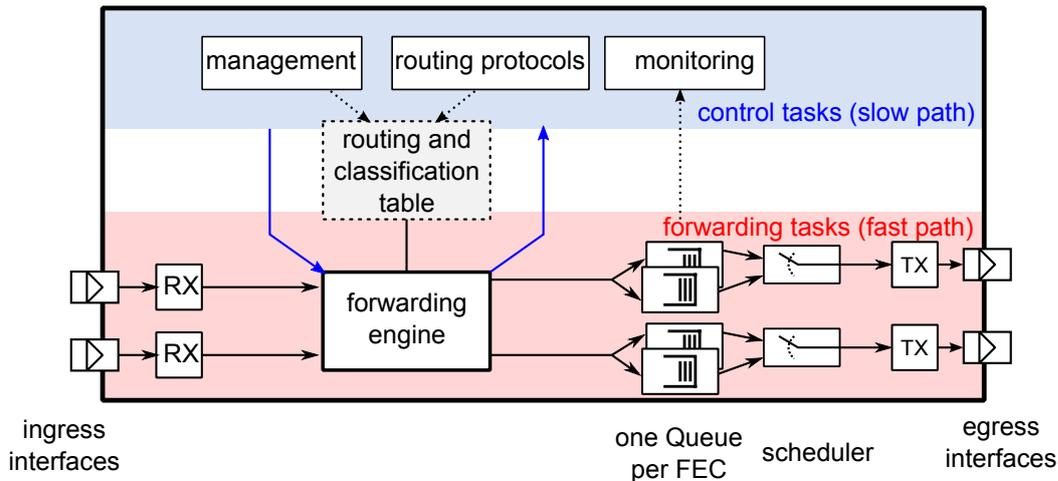
**Figure 2.3:** Router functions
