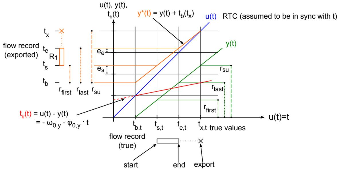
**Figure 4.16:** Impact of system time skew on record start and end timestamps
