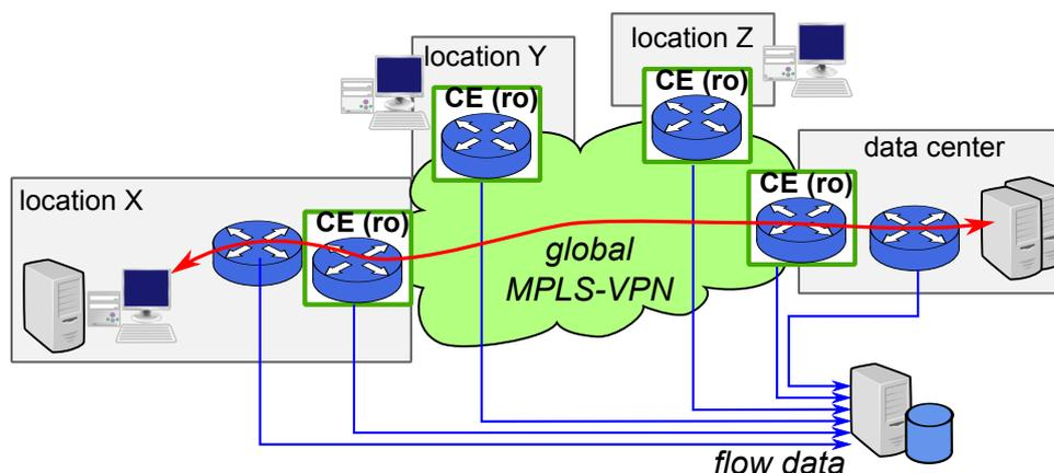
**Figure 3.17:** Typical flow capturing deployment in an enterprise network
