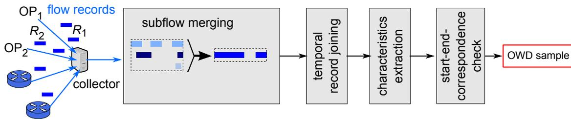
**Figure 4.12:** Extraction model extended with block for subflow merging
