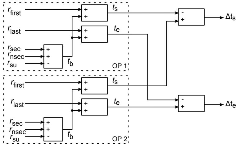
**Figure 4.20:** Measurement functions for OWD calculation
