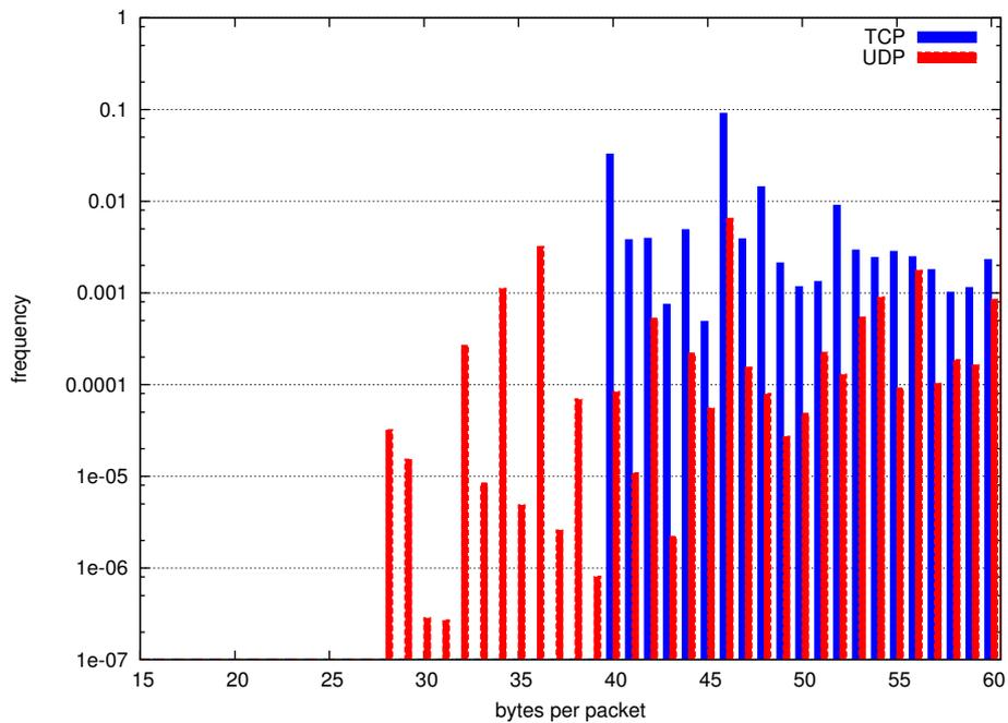
**Figure A.2:** Packet size distribution histograms from multi-packet-estimate for UDP and TCP flows with port number unequal to zero (no fragments). Truncated at 60 bytes, logarithmic Y-Axis.
