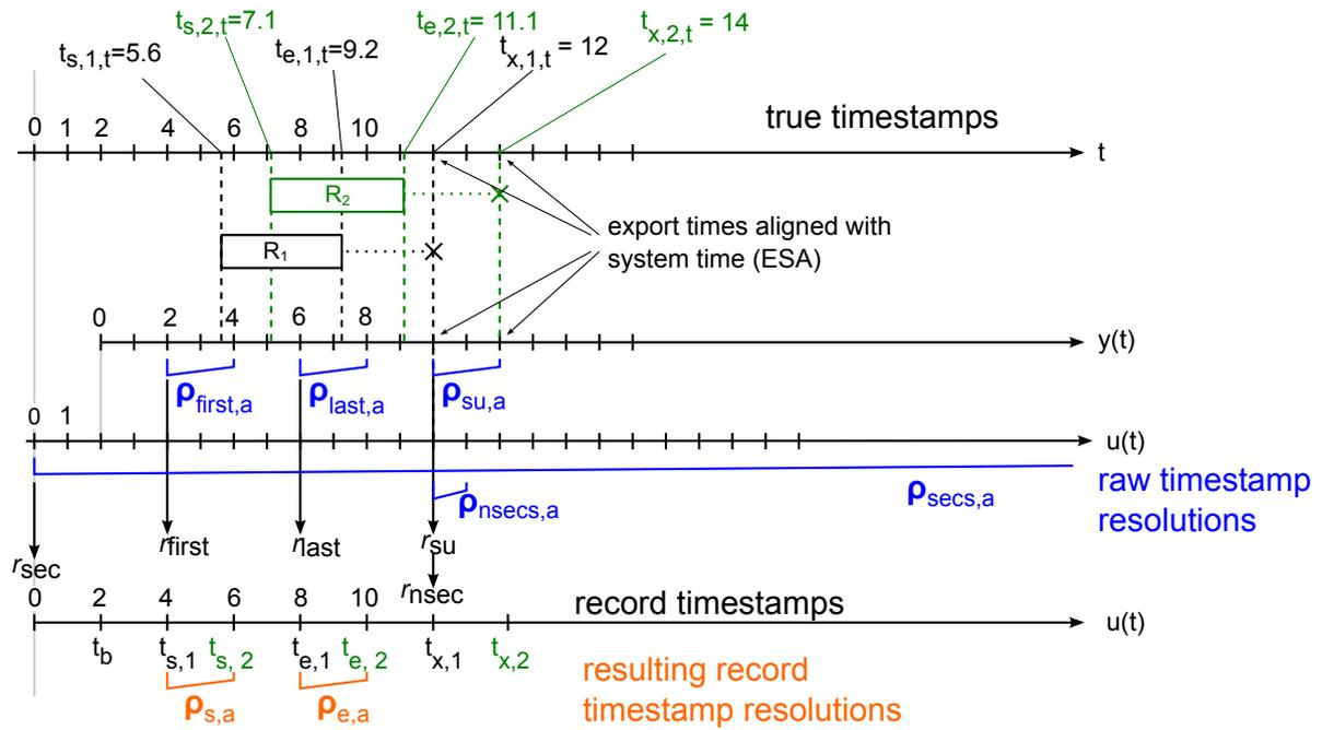
**Figure 4.18:** Illustration of timestamp resolutions (aligned timestamps)
