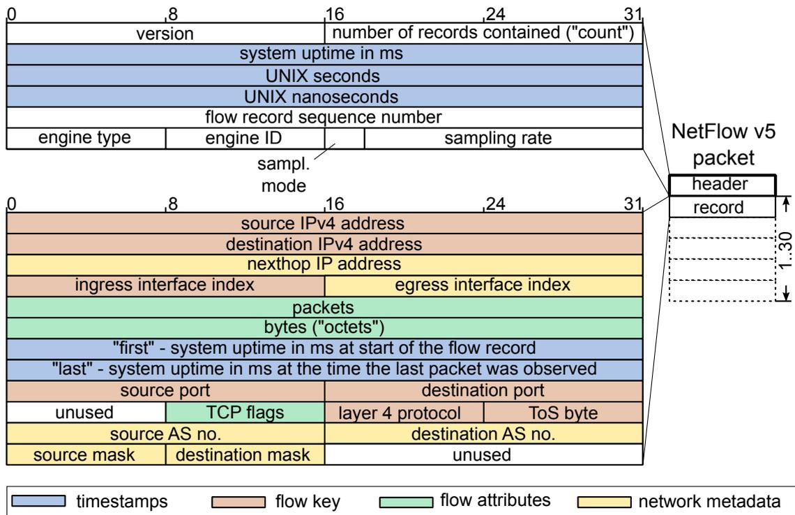
**Figure 3.11:** NetFlow version 5 packet format (header and record)
