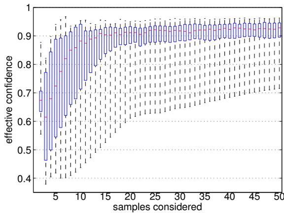
(a) Confidence interval calculated based on the Student-T distribution
