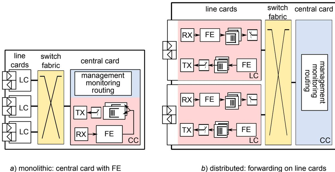
**Figure 2.4:** Router architectures
