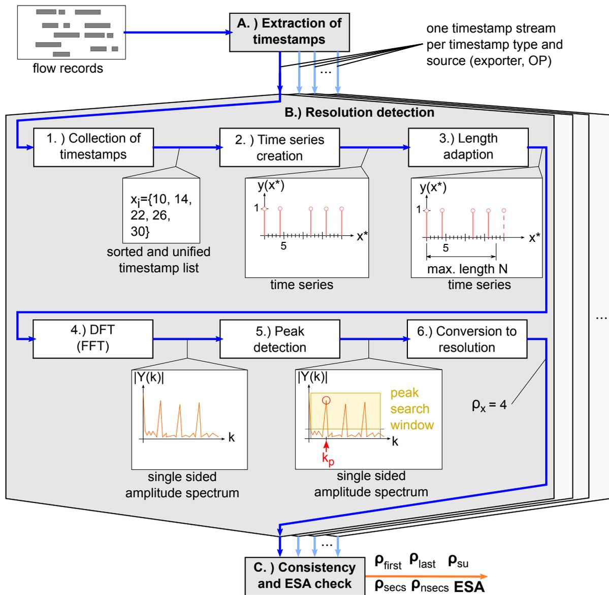
**Figure 6.3:** Resolution profiling procedure
