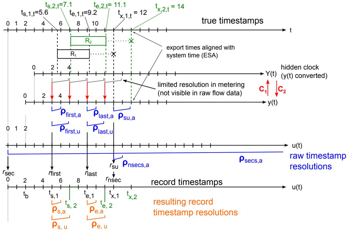
**Figure 4.19:** Illustration of timestamp resolutions, including conversion effects that lead to unaligned timestamps
