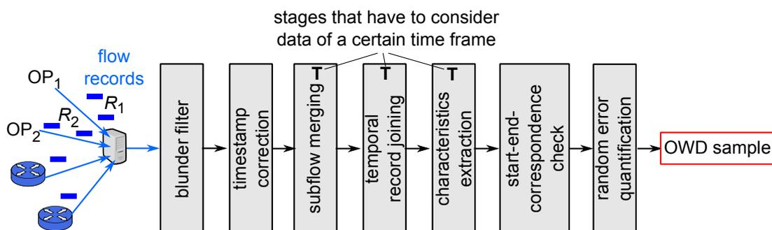
**Figure 5.2:** Extended extraction model indicating stages that have to consider data of a certain time interval
