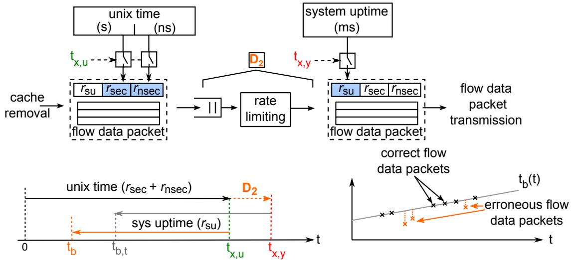
**Figure 4.24:** Error introduced by exporter-internal delay in the exporting process
