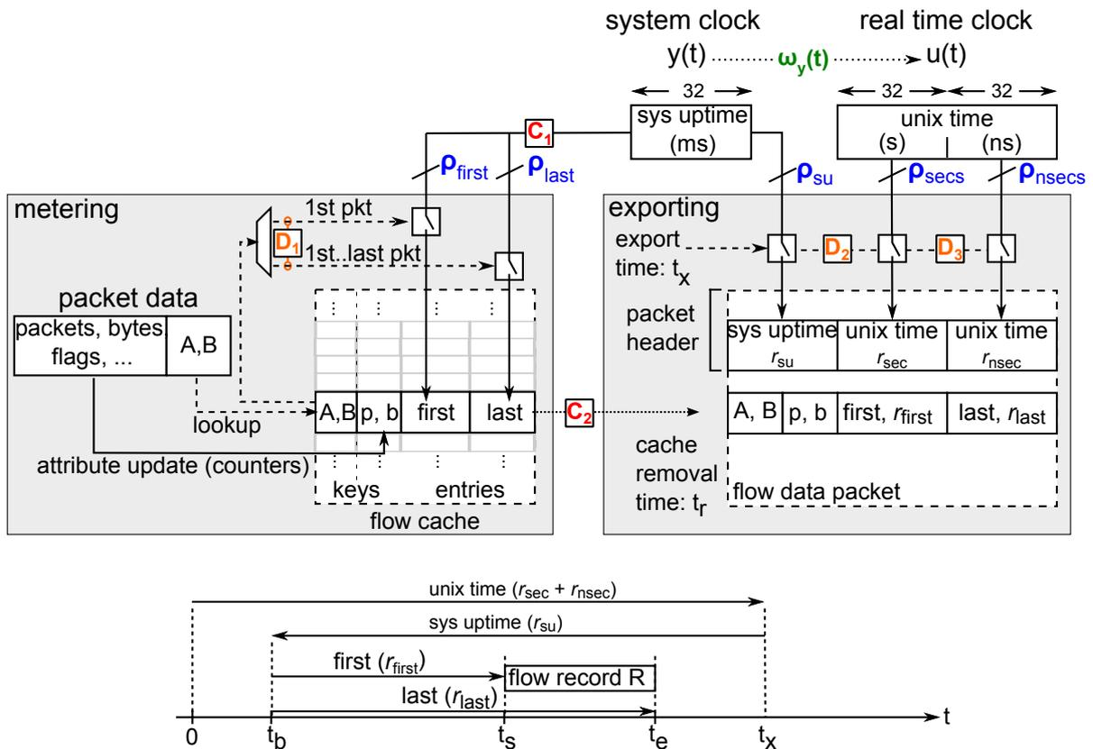
**Figure 4.15:** Timestamp creation model highlighting accuracy impacting points
