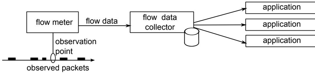
**Figure 3.3:** Flow capturing components
