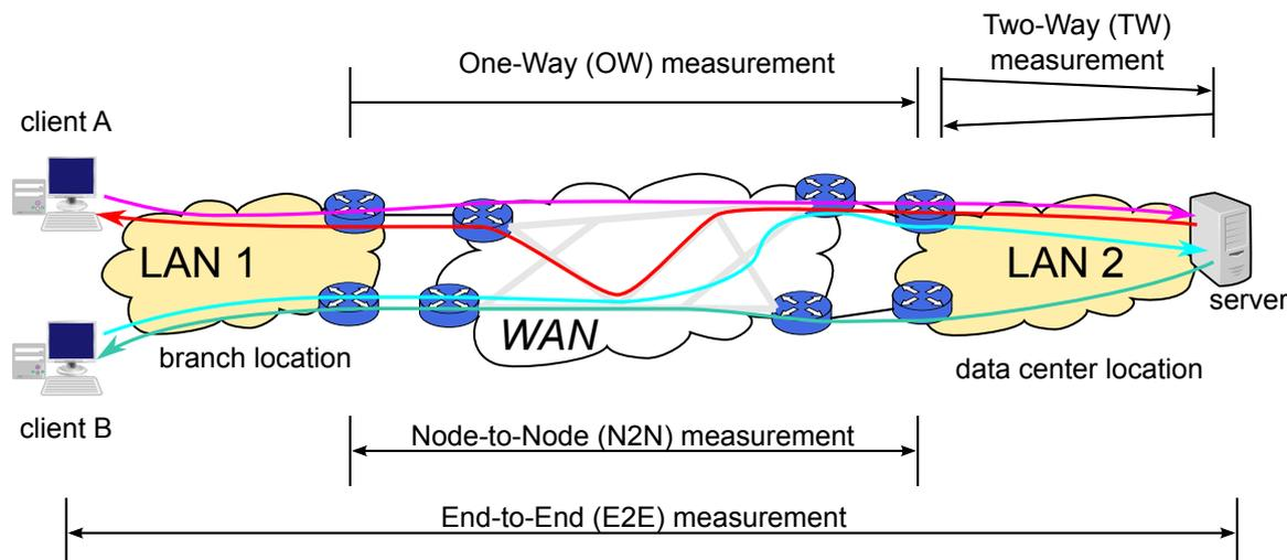
**Figure 4.1:** Traffic paths and measurement paths in an enterprise network
