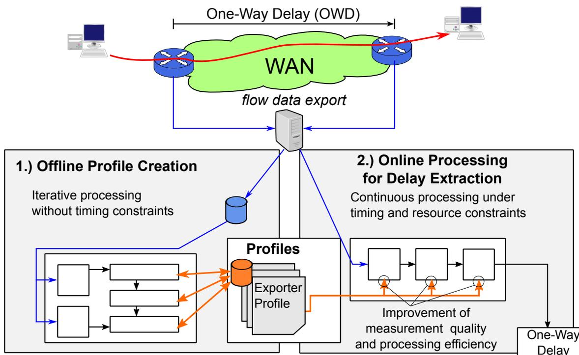
**Figure 1.1:** Overview of the flow-based OWD measurement method with profile support. It consists of the block for exporter profile creation (left) and delay extraction (right), which makes use of the previously obtained exporter profiles.
