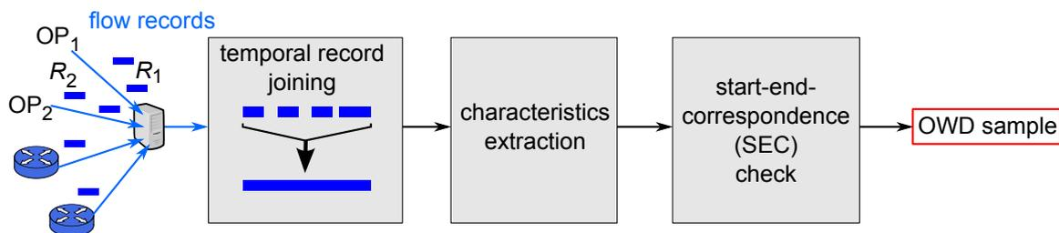
**Figure 4.9:** Extraction model extended for temporal joining of records
