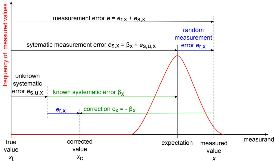
**Figure 2.7:** Illustration of measurement values and errors; based on [DIN 1319-1]
