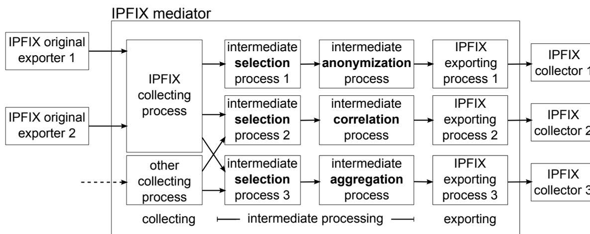
**Figure 3.18:** IPFIX Mediation Framework overview (based on [103])
