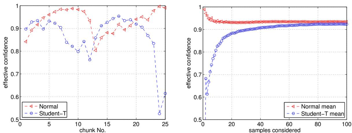
(a) Effective confidence for 15 samples per window over chunks (b) Mean values for window sizes of up to 100 samples
