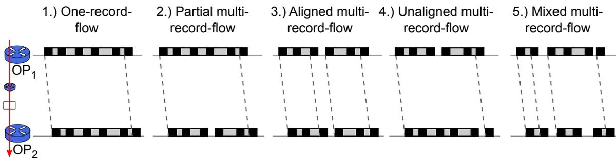
**Figure 4.8:** Flow record alignment
