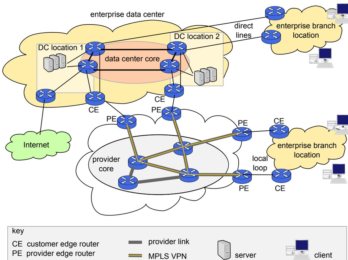
**Figure 2.6:** Enterprise network topology principle
