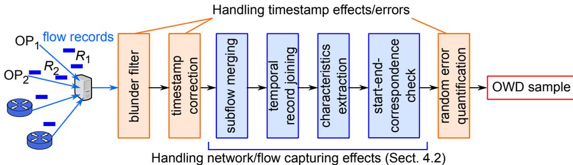
**Figure 4.26:** Extraction model extended for taking timestamp errors into account
