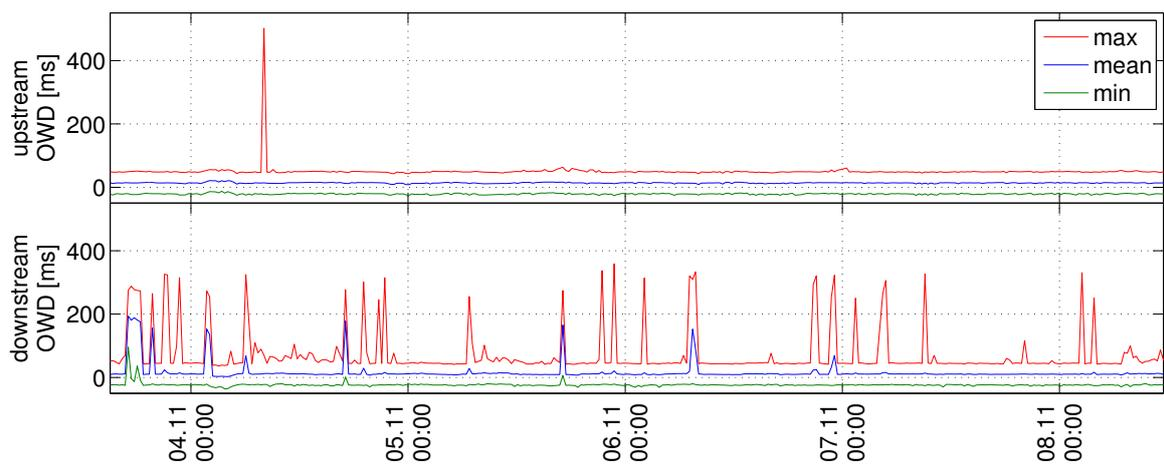
(c) Corrected flow-based OWD of RTT measurement traffic
