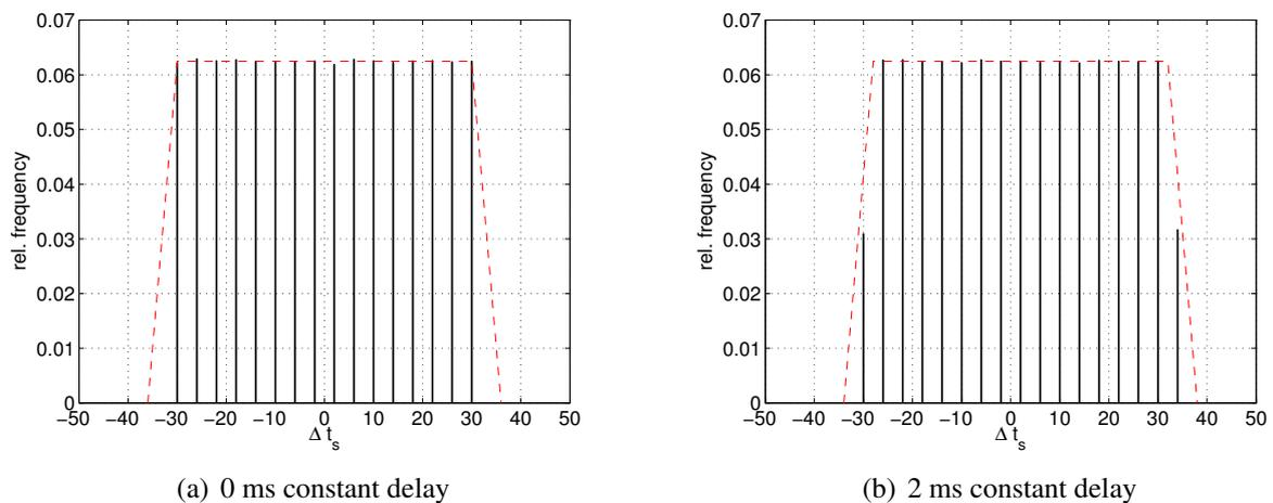
**Figure B.1:**  $\Delta t_s$  distribution from Monte Carlo experiments. Random error characteristic for an OPP with  $\rho_{s,OP1} = 4 \text{ ms}$ ,  $\rho_{s,OP1} = 64 \text{ ms}$
