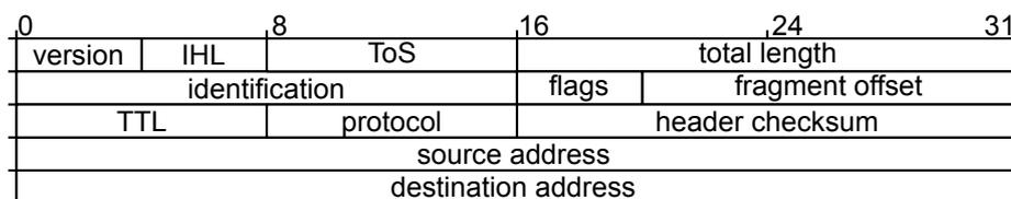
**Figure 2.1:** IPv4 header format
