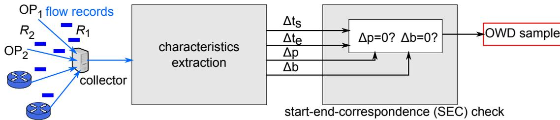
**Figure 4.7:** Extraction model extended by the SEC check block
