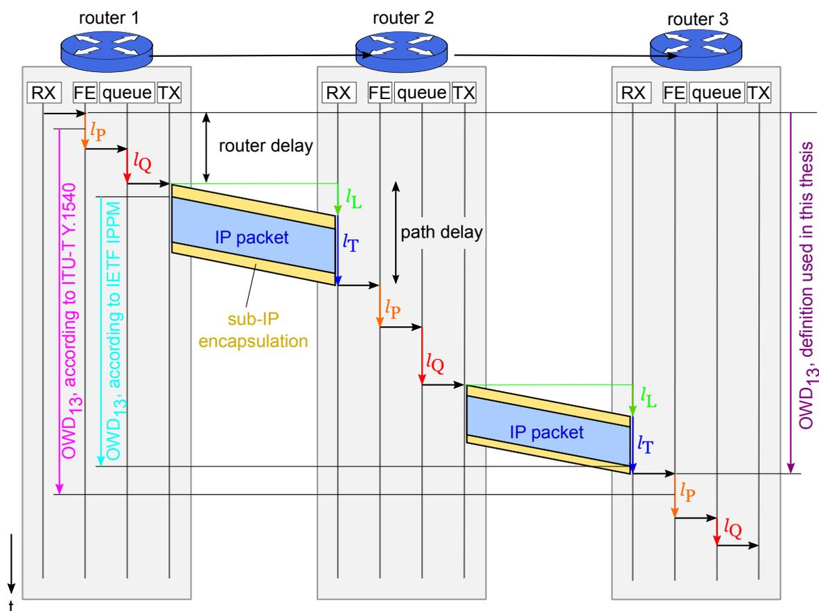
**Figure 2.9:** One-way delay definitions
