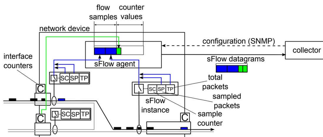
**Figure 3.9:** sFlow statistical packet sampling
