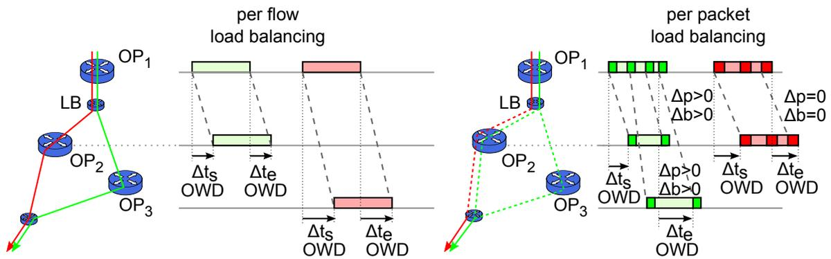
**Figure 4.6:** Effects from load balancing
