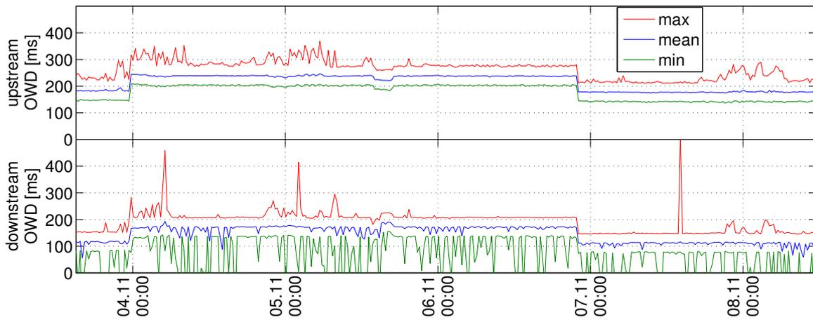
(b) Uncorrected flow-based OWD of RTT measurement traffic
