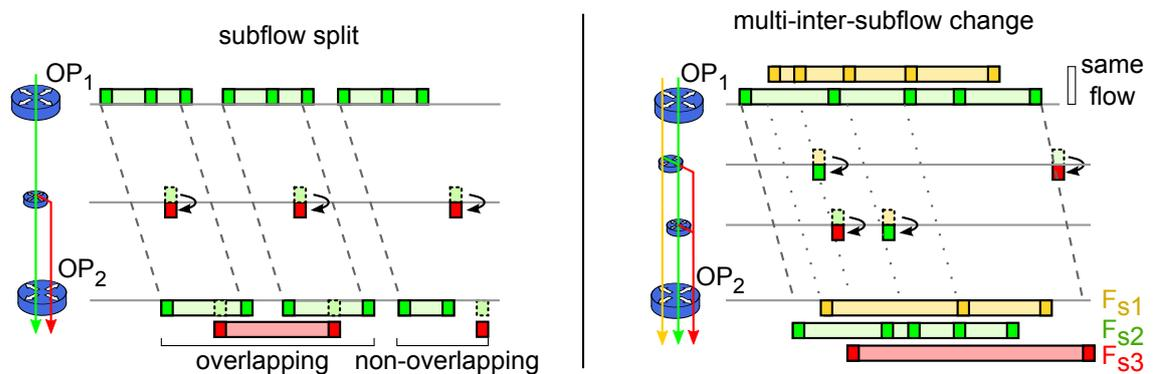
**Figure 4.11:** Effects of path variant fields in the flow key with partial subflow change
