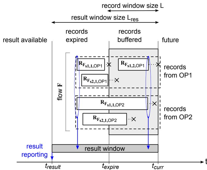
**Figure 5.6:** Window containing subflows of a multi-record-flow that require joining and merging
