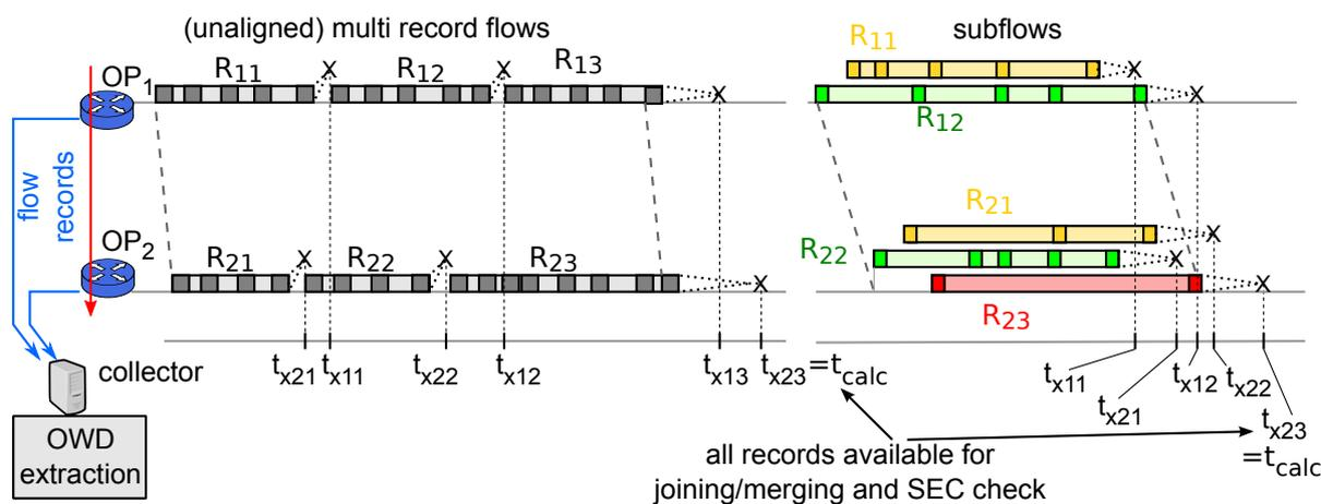
**Figure 5.1:** Impact of multi-record-flows and subflows on delay extraction time
