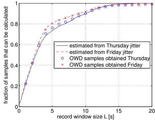
**Figure 7.11:** Samples calculated from per-OPP export jitter PDFs compared to samples obtained using different record window sizes
