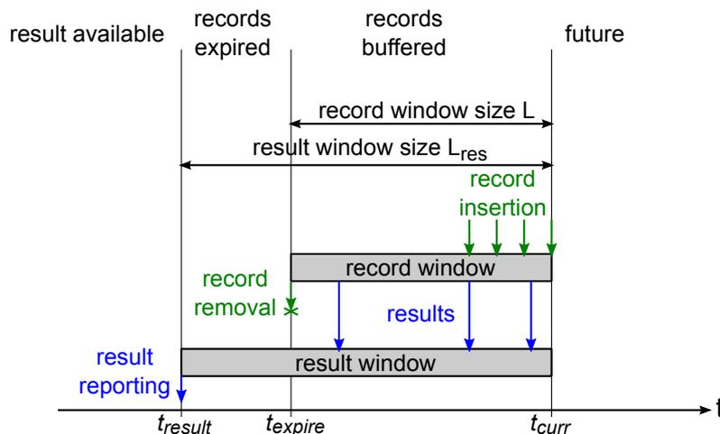
**Figure 5.3:** Window-based OWD extraction principle
