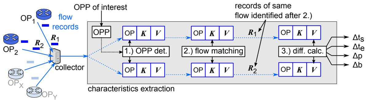
**Figure 4.3:** Characteristics extraction model
