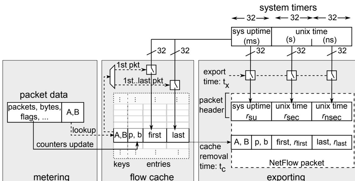
**Figure 3.12:** Model for NetFlow flow capturing and timestamp creation
