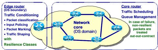
Figure 2: RD-QoS signaling with DiffServ
