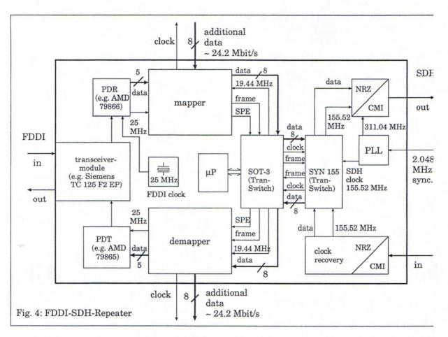
After the FDDI transceiver module, the incoming FDDI bit stream of 125 Mbit/s is transformed by the FDDI Physical Data Receiver to symbols of 5 bit at a symbol clock rate of 25 MHz and fed into the mapper circuit.
