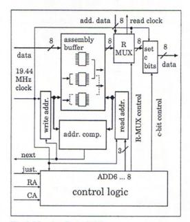
Fig. 6: Mapping Control Unit
