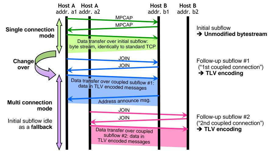
→ Payload encoding outside initial subflow (used also for fallback)
