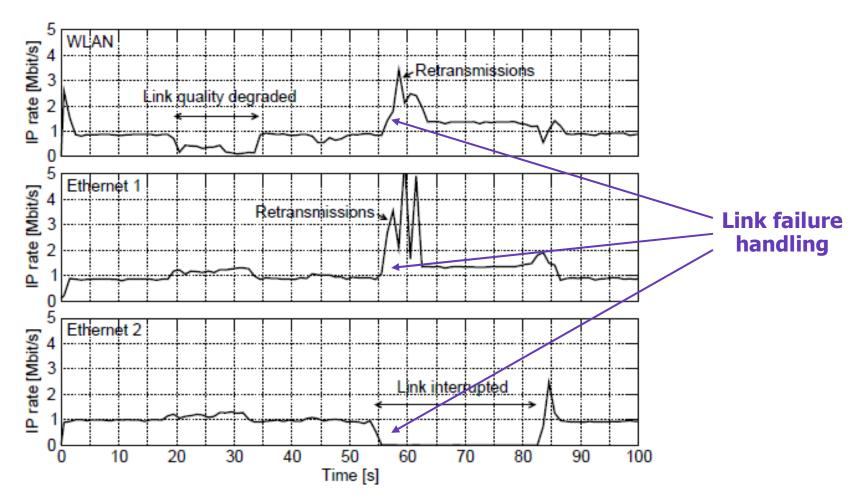
→ Compensation of path failures transparent to applications
